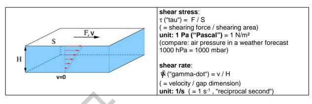
This theory is applicable with "Laminar flow" conditions. We consider that liquid is composed of many layer, who move at different speed each other. But this "Laminar Flow" exists only for small distance (H on figure above), directly in contact with mobile. This is why DIN measuring system should be uses always with adapted cup (cylinder) or small gap (cone and plate).
