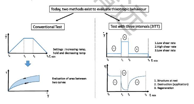
Interest of 3ITT test is to get information about time to recover viscosity after application. But for this two methods, best is to use DIN MS.
